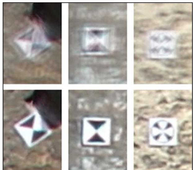
Figure 10. Corresponding orthoimages patches, from 7 images, without (above) and with (below) correction of lens distortion.
