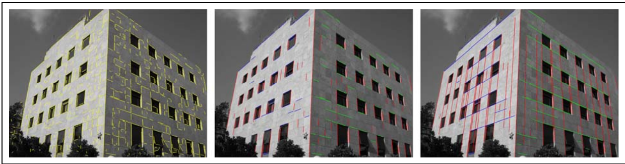
Figure 8. Initial extracted edges (left), line segments grouped in dominant vanishing points (centre) and final segments (right) after correction of lens distortion [last image in Fig. 6].
