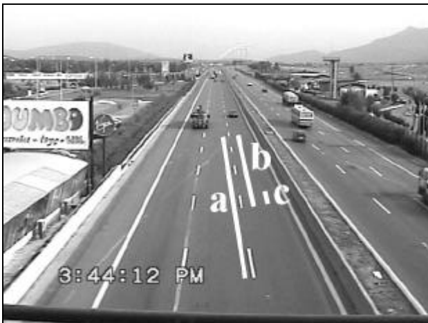
Figure 10. Known distances a, b, c used for speed estimation.
